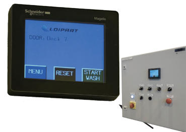
Fig. 3: Main chute control system
